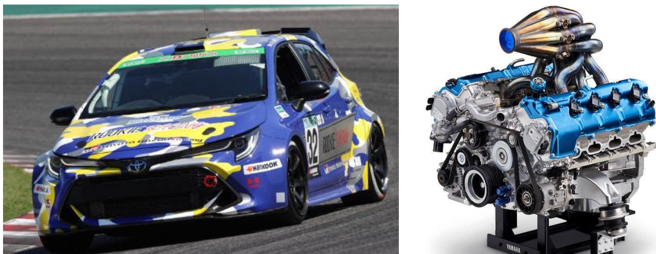
Figure 4. Toyota Corolla with a hydrogen engine and Yamaha V8 hydrogen unit [4]
