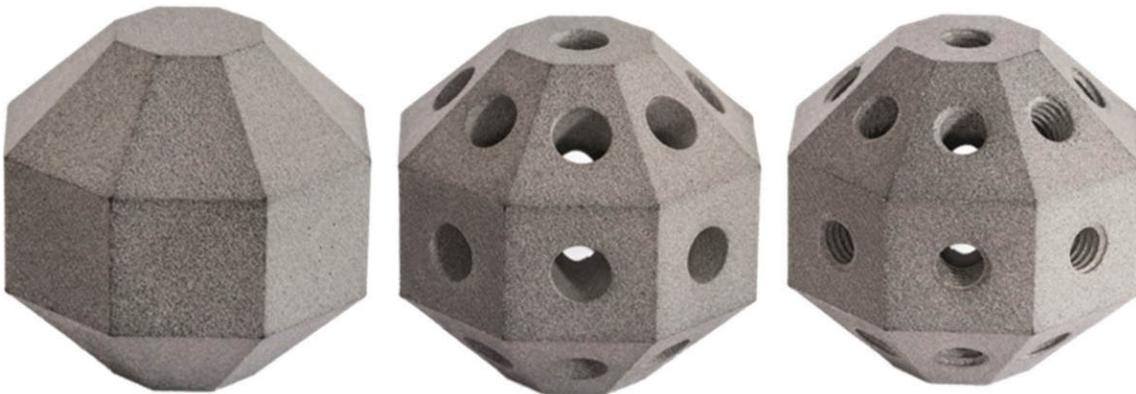
**Figure 6.** Realistically created identification experimental samples and their three variants plan P, with holes D and Z threads produced by MJF technology
