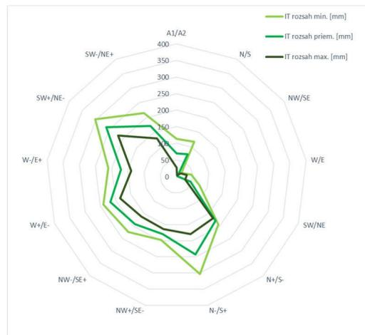
**Figure 16.** Summarizing the values from measurements for MJF technology, the shape of the sample with Z threads, and their graphical comparison in the polar view
