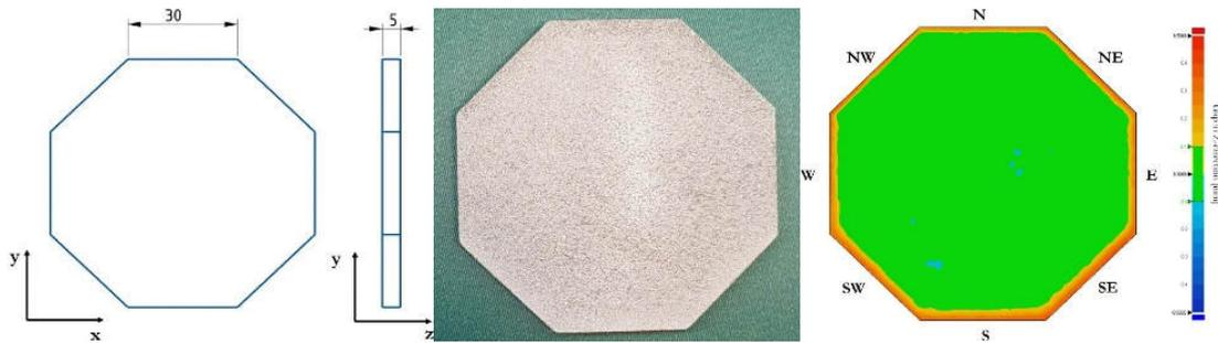
**Figure 2.** Benchmark geometry, a manufactured benchmark part (upper surface), and map of deviations of the upper surface along the Z-axis. (12)
