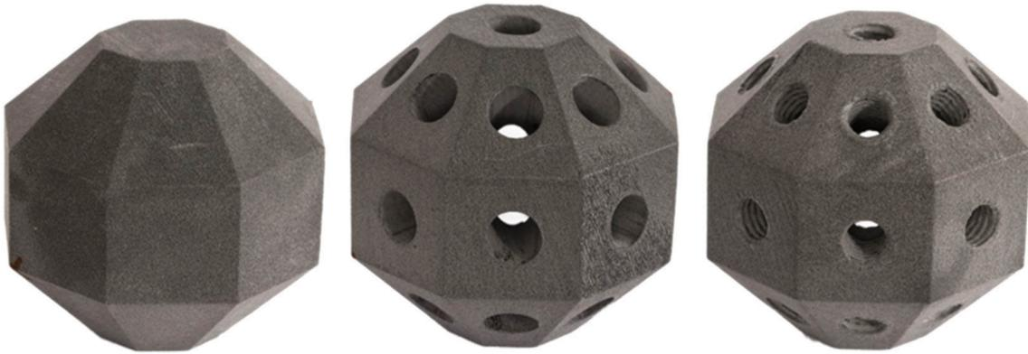
**Figure 5.** Realistically created identification experimental samples and their three variants plan P, with holes D and threads Z produced by SLS technology
