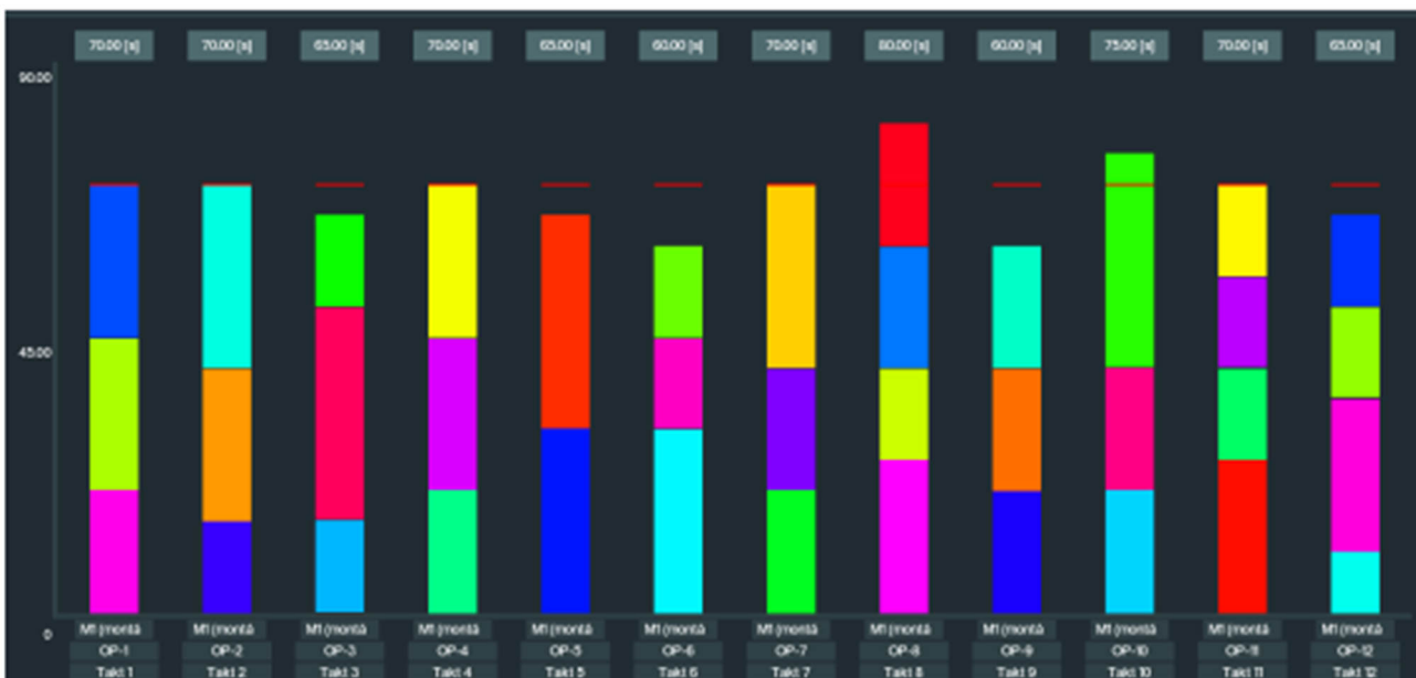
Figure 11. Demonstration of the state of the assembly line after redistributing the operation and creating an optimal design [Source: Authors]
