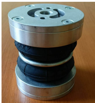
Figure 2. Flexible pneumatic element.
