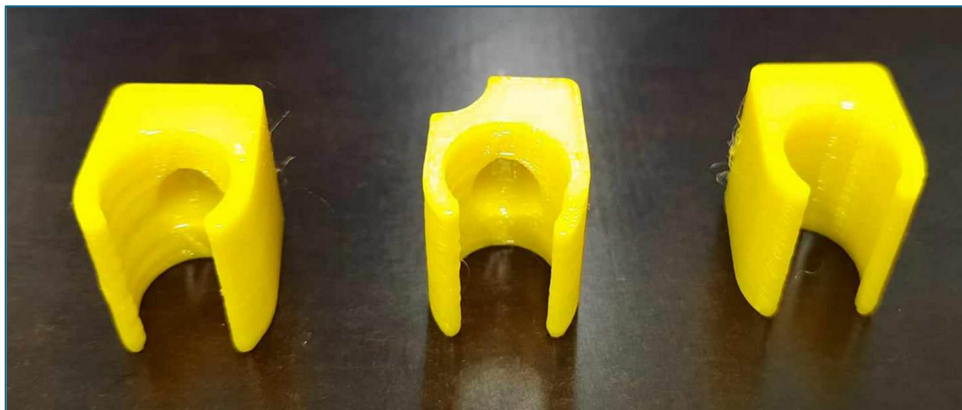
Figure 9. Cable holder models produced with the FDM method using a 3D printer
