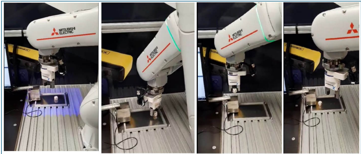
Figure 3. Cobot work cycle in a pick-and-place application
