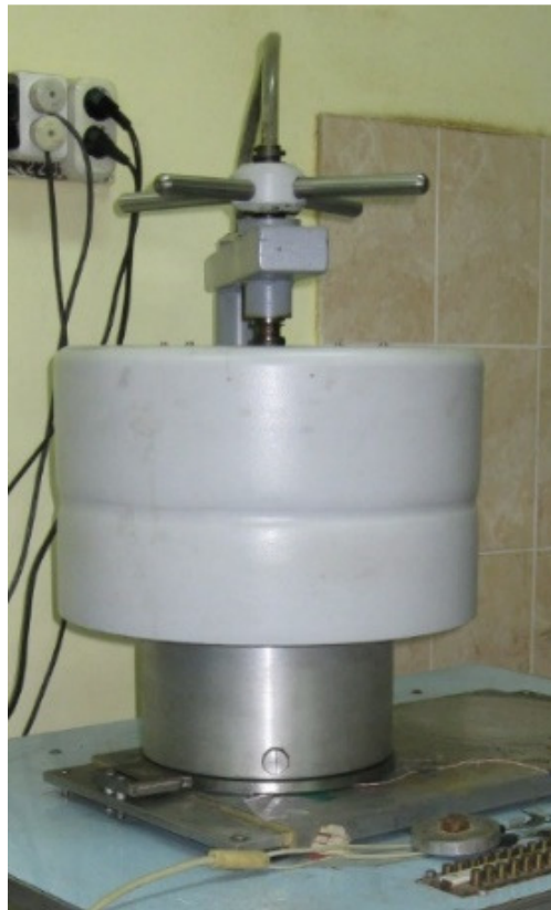
Figure 8. Measurement System RGU-2 for calibrating the heat flux sensors and measuring the emissivity of coatings and material surfaces
