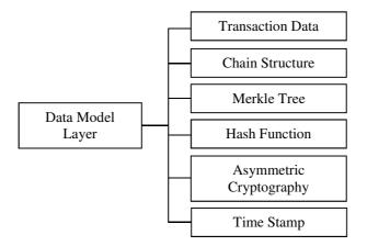
Figure 3. Main components of the data model layer of Blockchain architecture
