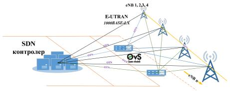
Figure 1. Architecture software-defined networking
