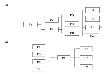
Figure 4. Breakdown into serial / parallel model blocks for calculating mobile network reliability: a –the scheme is a decentralized IP network; b - centralized SDN network
