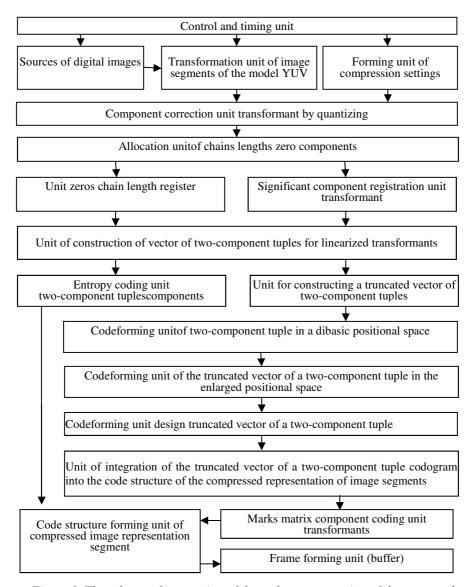
Figure 1. The scheme of integration of the code representation of the truncated vector of two-component tuples into compression technology on the JPEG platform
