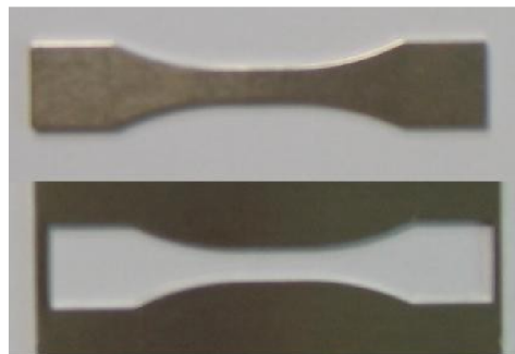
Figure 6. Photo of the specimen using a blanking process and a blanked-out plate.
