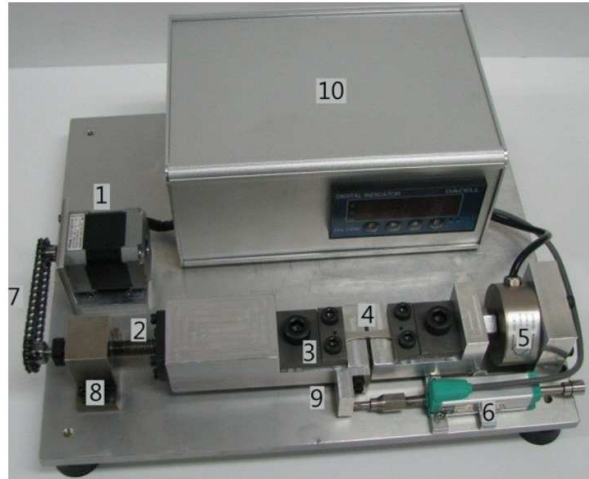
Figure 1. Photo of the miniature tensile testing machine with a size of 330 x 280 x 155 mm: 1) stepping motor; 2) ball screw block; 3) specimen holders; 4) miniature tensile specimen; 5) load-cell; 6) displacement gage; 7) chain; 8) bearing holder; 9) linear motion guide; and 10) control box.
