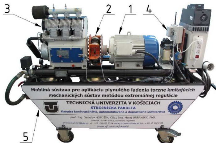
Figure 1. The newly build mobile torsional oscillating mechanical system
