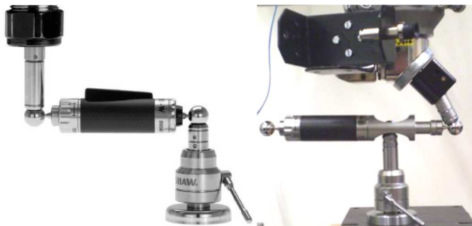
Figure 2. Renishaw Ballbar QC20-W and its mounting on effector of delta robot Fanuc M-1iA [8]
