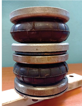
Figure 1. A pair of flexible elements connected by a connecting flange
