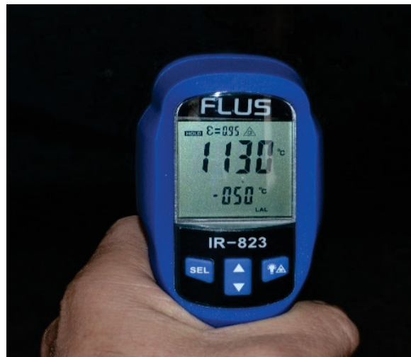
Figure 2. Results of temperature measurement at the gas injection nozzle
