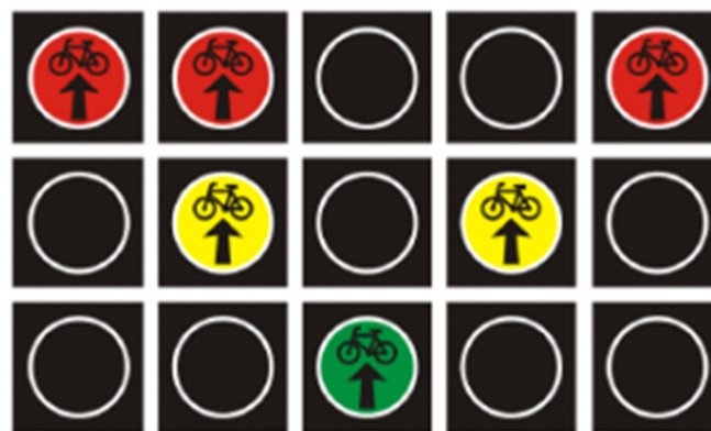
Figure 3. Directional signal for cyclists [5]
